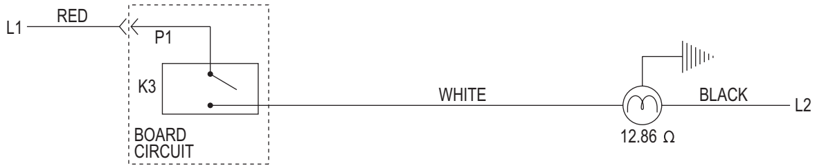
Door Latch Motor Strip Circuit
